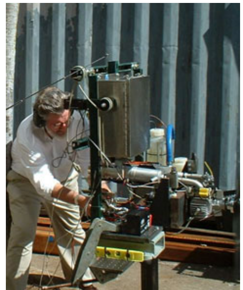
Dr. John Langley tests a thermoelectric generator for a heavy-fuel unmanned aerial vehicle engine
